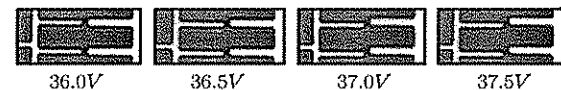
Fig. 2 Microscope snapshots of a pair of combfingers ( V_0 shown below each image). Their relative position demonstrates the buckling event.
