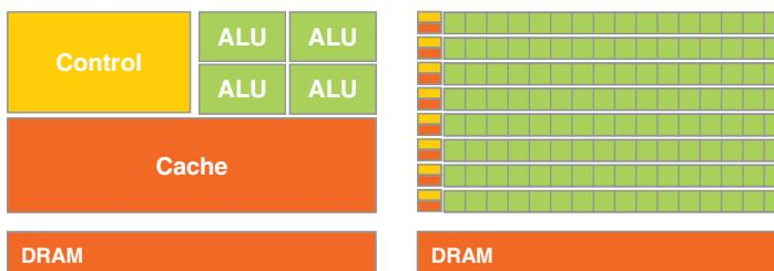
Figure 1. CPU vs GPU architecture. There are more transistors devoted to data processing rather than to data caching and flow control for the GPU, compared with the CPU.
