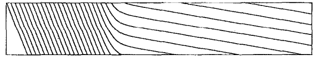
FIG. 13. Base-state streamfunction contours in a stationary reference frame where U=1 and (V_1, V_2) = (-4.5, -0.3) . Stretching of the interface due to the base-flow velocity field causes persistent steep gradients at the root of the finger.
