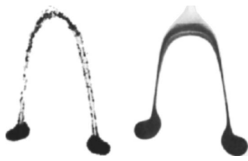
FIG. 7. Disintegrated suspension drop (left) and liquid drop (right) in an experiment by Machu et al. (Ref. 9).
