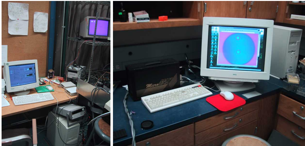
Figure 5.16: View of data acquisition PC (left) and digital image processing PC (right), including camera controller.
